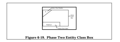
To get started on this effort requires that the modeler become intimately familiar with the basic structural figure of modeling-the entity class box. A sample is shown in Figure 6-19. The symbol of an entity class is a simple rectangle with a small rectangle in the lower left hand corner for the entity class label, and a small triangle in the upper left hand corner for the entity class number.
